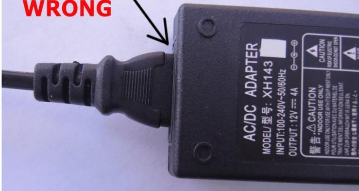
Plug all the way into the AC/DC Adapter
