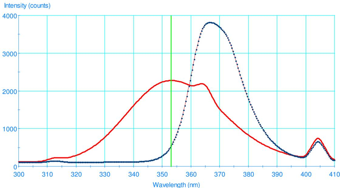
Figure A. Spectral Distributions of two UV SYSTEMS, Inc. TripleBright LW lamps without any LW filters.
