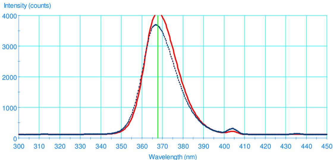
Figure D. 300 to 450 nm Spectral Distributions of a Philips and GE BLB LW370 lamps.
