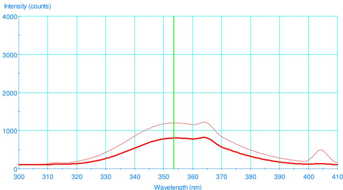
Figure C. Spectral Distributions of a UV SYSTEMS, Inc. SuperBright LW lamp with and without the FL-20 LW filters. Top curve is a LL-16-351 and the bottom is the same lamp but as measured through a FL-20 LW filter. The scale is the same as Figure B.
