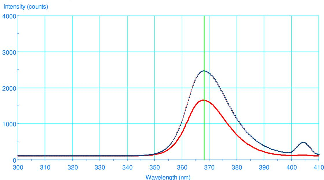
Figure B. Spectral Distributions of a UV SYSTEMS, Inc. SuperBright LW lamp with and without the FL-20 LW filter.
