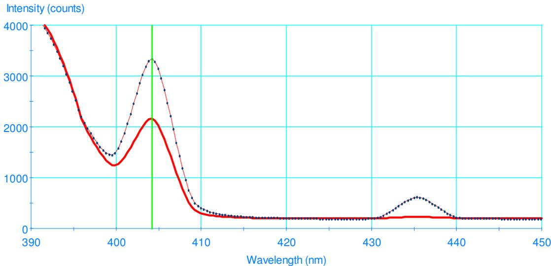
Figure E. 390 to 450 nm Spectral Distributions of a GE vs. Philips F20T12/BLB LW370 lamps.
