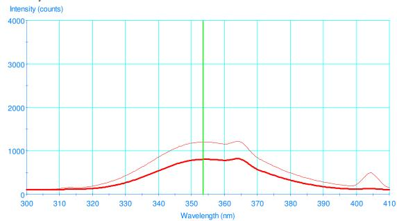
Peak wavelength is 352 nm (OO says 353.50 nm). Same lamp WITHOUT and with the LW filters. Measured on 11/10/02 by DEN.
